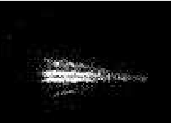
Fig. 2. Image of a few \alpha -particle tracks recorded with a low-noise CCD device. The exposure time is 0.1 s.
